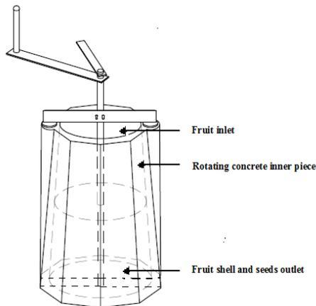
Figure : side view of the Universal Nut Sheller
