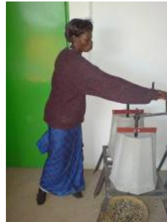
Figure 2: Universal Nut Sheller [1]
