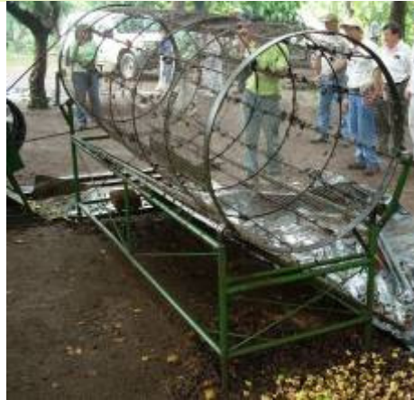
Figure 6: sketch and photograph of a separator in operation (used in the Gota Verde project in Honduras). When shells and seeds of dry fruits cannot be separated easily, they should be separated with a blower or when no power is available in the field, by wind.
