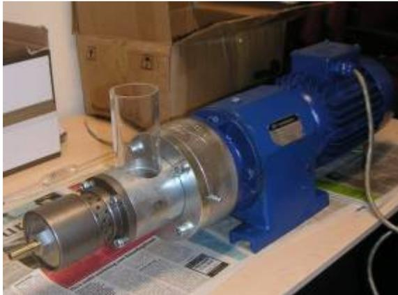
**Figure 6** – The Danish BT press is an example of a cylinder-hole type press. Notice the nozzle, left in front [10].
