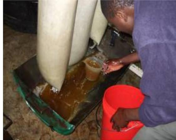
**Figure 11** – Left top: SVO filtration of cooking oil on the site of German supplier Monopoel. Right top: simple filtration setup using bag filters [picture Diligent Tanzania Ltd.]. Left bottom: improved setup for bag filters [picture Diligent Tanzania Ltd.]. Right bottom: employee collecting an oil sample for analysis after filtration [picture Diligent Tanzania Ltd.]
