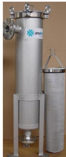
**Figure 19** Filter housing with filter basket from [www.amafilter.nl](http://www.amafilter.nl). The filter bag is inserted in the basket and need cleaning every 14 days.
