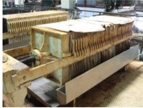
**Figure 15** Plate filter for food industry, capacity around 1000 liters/hour.
