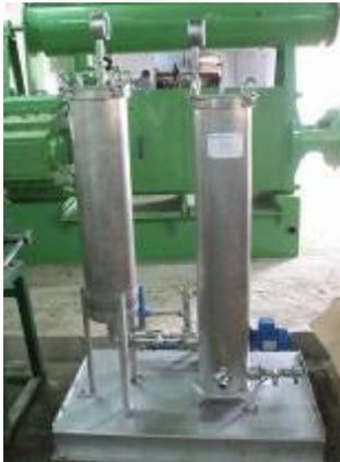
**Figure 20** Combined setup of a bag and candle filter form amafiltergroup. [picture Diligent Tanzania Ltd.].
