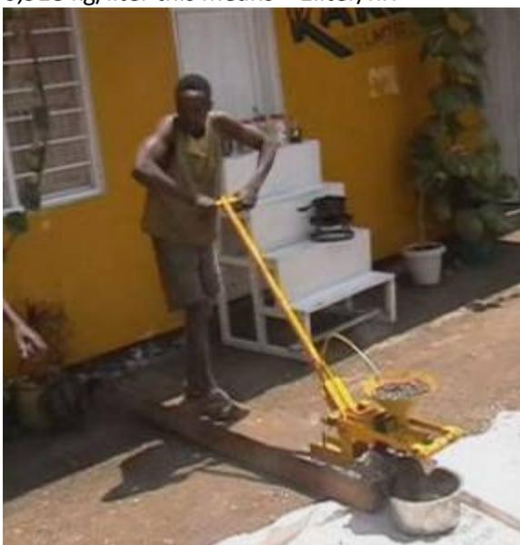
**Figure 2** – the Bielenberg ram press operated at Kakute Ltd., Tanzania [12]
