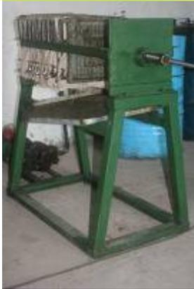
**Figure 14** Plate filter with capacity of 150 liters/hour. At Diligent Tanzania Ltd. Produced by TEMDO Tanzania.
