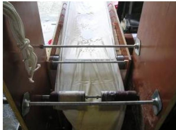
**Figure 13** Band filter in operation. The transport rollers are equipped with sandpaper for better friction. The cloth is continuously moving. [5].
