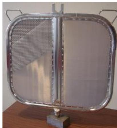
**Figure 17** Close-up of one of the filter plates. The framework around the mesh is made of hollow
