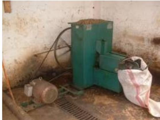
**Figure 7** – The Sundhara oil expeller is a representative of the strainer type presses. On the right side the choke adjustment. [12]
