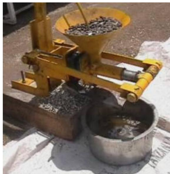
**Figure 3** – close-up of the Bielenberg pressing mechanism. Notice the automatic discharge of
