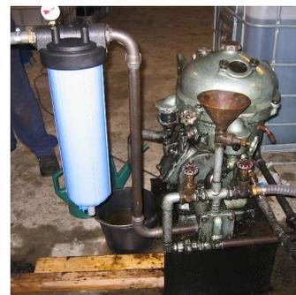
**Figure 24** - Example of a centrifugation system with a bag filter as a security [12].
