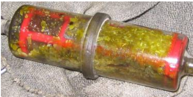
Figure 5.8 The photo shows an inline pre filter which was partly blocked by small particles of solid fat, released from a small piece of zinc coated steel in the PPO tank.
