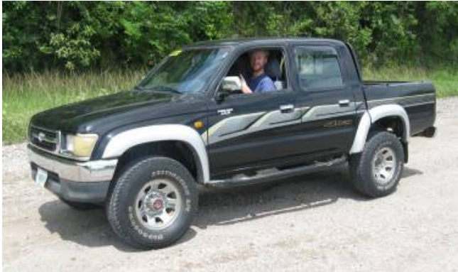
Figure 5.12 Toyota Hilux 2,8D (3L). IDI engine. Converted by an ELSBETT 1-tank system, Honduras October 2008 (Gota Verde Project).
